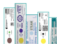
Figure 2. The chemical indicators used in this study. Three Type 6 (formally Class 6) and two Type 5 (formally Class 5)
