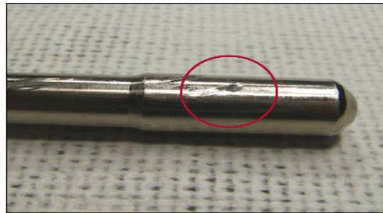
Drill Guide Sleeve: scratches on the surface
