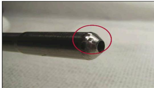
Drill Guide Sleeve: dents on the sleeve tip
